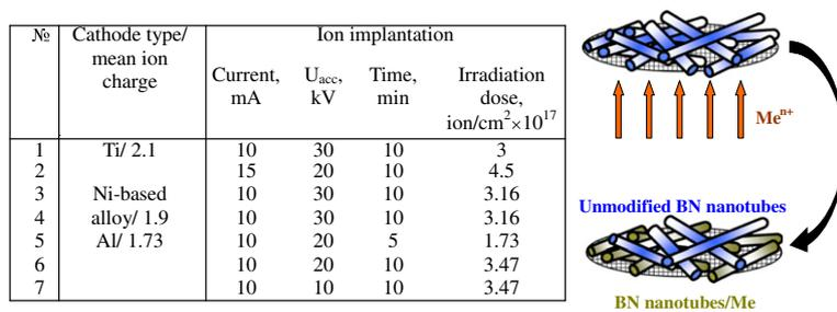
Figure 1. Ion-implantation parameters and schematics of high-energy ion modification of BNNTs during ion implantation.
